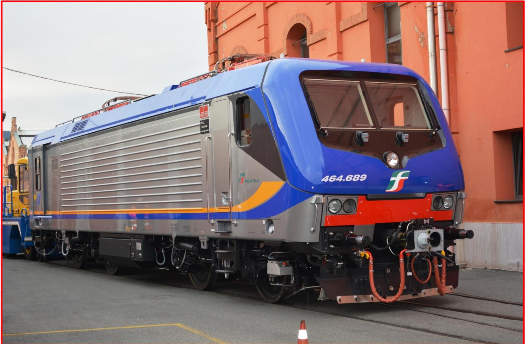
**Loco E412 / EU43 – 3 kV DC / 15 kV 16 <sup>2</sup>/<sub>3</sub> Hz**
